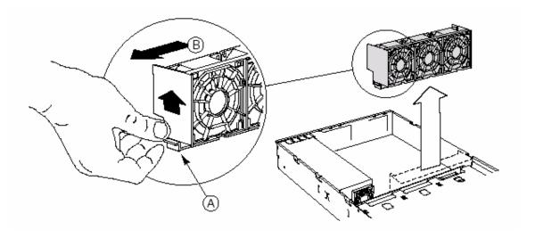
Figure 10: Removing the Fan Assembly
